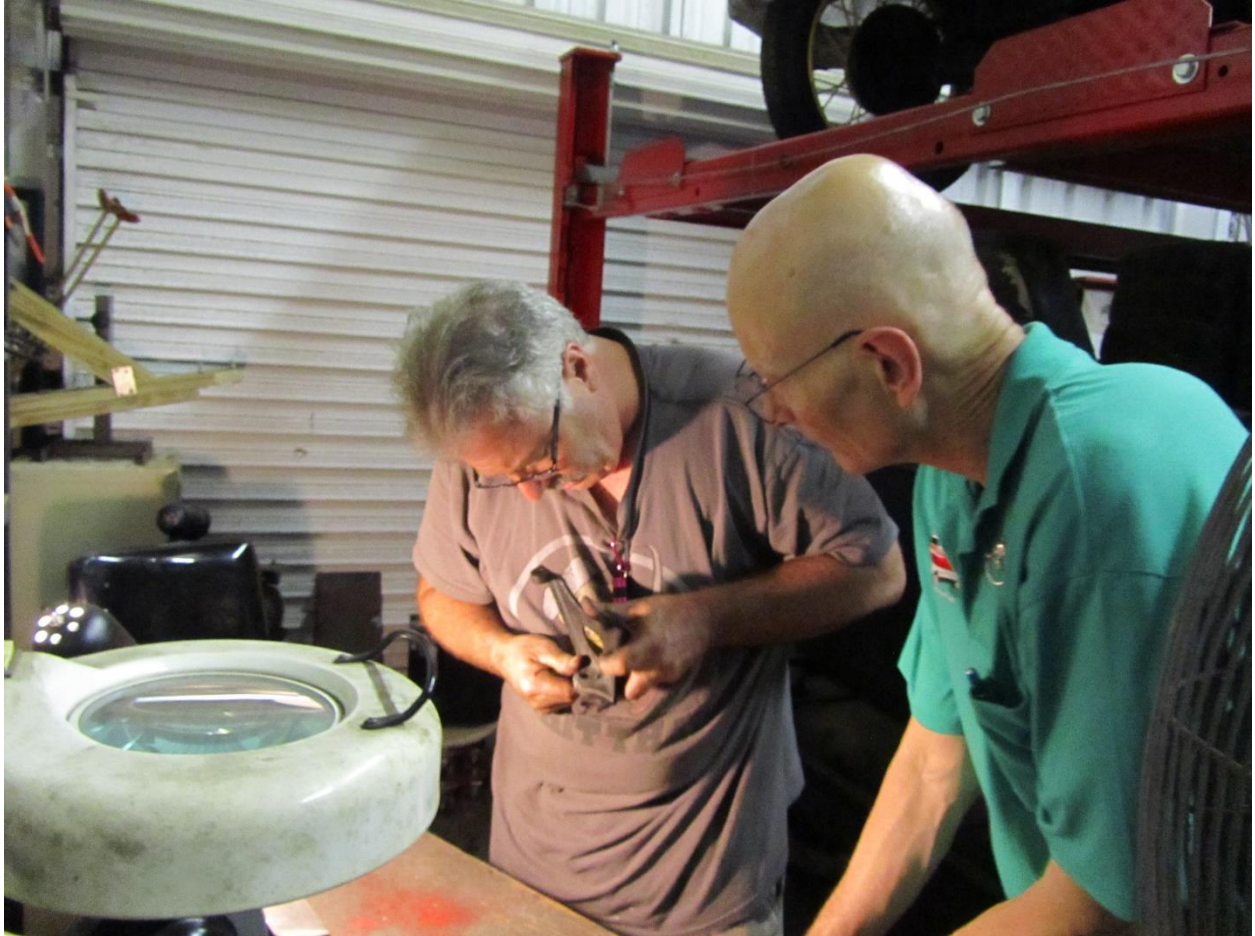
The first alternative was to remove the pump mounting bracket and begin grinding to alleviate some of the clearance issue. Paul and Norm work on the bracket above.
